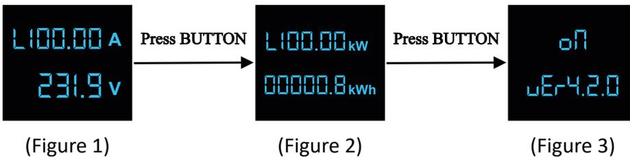
3.2 Single phase two way monitoring module(AC)
