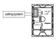
The switch provides a group of Normally Open contact (NO) and a group of Normally Close contact (NC) ,COM is connection common terminal.
