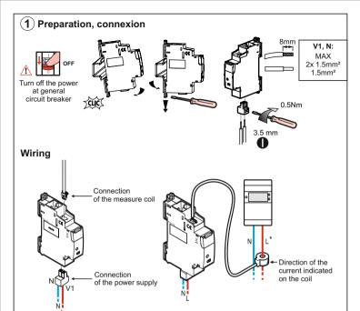
A circuit breaker with rated current C2 to C16 is necessary depending on wire section used for supplying the energy meter.
