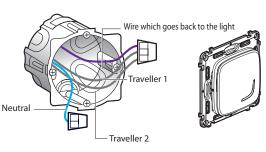
Use a connector to connect all 3 wires together (travellers 1 and 2 and lamp return wire). Use an other connector for neutral wire.
