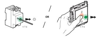
To complete your installation, briefly press the configuration button of the **Control Modul** or in the middle of the **wireless master switch**.
