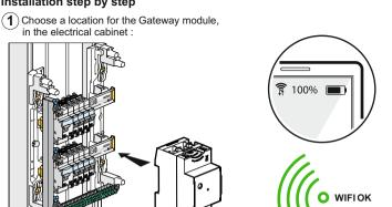
If an internet box is present in the house, check with a smartphone that the Wifi signal level is sufficient. If the signal is not enough, try to bring the internet box to the electrical panel or add a WiFi repeater at the installation
