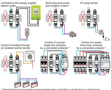
\*: Non-functional consumption measurement when controlling a single line or a three lines power contactor by a connected contactor.
