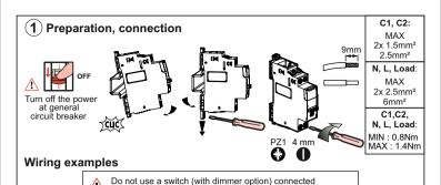
The control circuit (upstream terminals C1 and C2) have an integrated power and an integrated protection.
