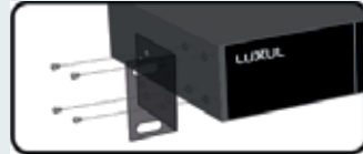
Install brackets for rack-mounting
