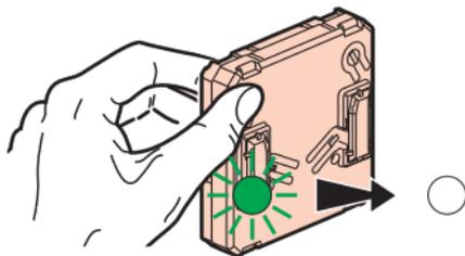
**Briefly** press on a button of the transmitter to activate it. The indicator lights will flash green and then switch off.
