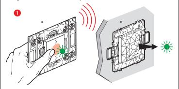
Press the centre of the **wireless master switch** until the indicator lights up in green, release and the indicator will go off.
