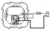
2 commandes d'éclairage / 2 controls lighting circuit
