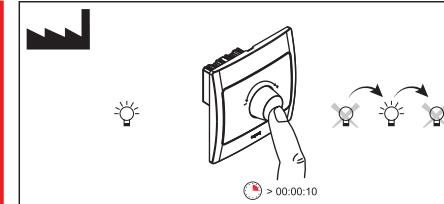
When the lamp is ON, push the Button, the lamp will turn OFF, continue holding for 5 seconds, then the lamp will turn ON again --> Continue for 5 seconds --> The lamp will turn OFF, the system has reset to the default value.
