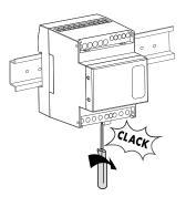
For fastening the device on the DIN rail: 5,5 mm flat screwdriver (from 4 to 6 mm).
