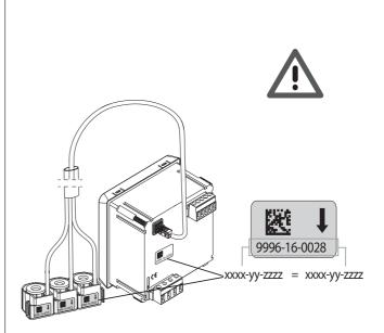
The combination of the code on the coils and on the instrument guarantees the perfect calibration of the two and guarantees the measurement class.
