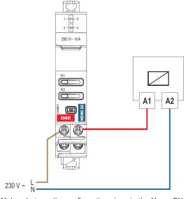
**Note:** whatever the configuration given to the Nemo SX Multifunction control module, local command of the module is still possible pushing on the 2 buttons on the front face of the module;
