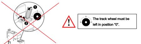
. It is not necessary to address the Nemo SX modules. The track wheel must be left in default position "0".
