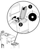
In this system the Modbus address of a Nemo SX Nemo SX module device or group of modules (several functions) is obtained considering the address of the interface Modbus/Nemo SX Interface as tenth and the address of a device or group of function as unit (e.g. Interface address 1 =  $10 \rightarrow$  address of module n°5 = Modbus address 15)
