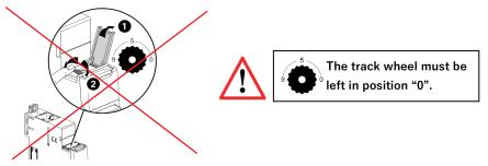
. It is not necessary to assign an address via rotary; **The track wheel must be left in default position "O**".
