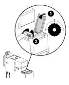
. Marked from 0 to 9 in order to locally define the Modbus address to Nemo SX modules In this system the Modbus address of a Nemo SX Nemo SX module device or group of modules (several functions) is obtained considering the address of the interface Modbus/Nemo SX Interface as tenth and the address of a device or group of function as unit (e.g. Interface address  $1 = 10 \rightarrow$  address of module n° 5 = Modbus address 15)
