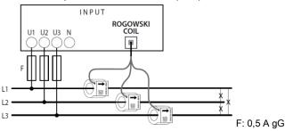
4 wires three-phase network, 3 sensors (3N-3E):
