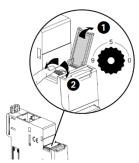
. Marked from 0 to 9 in order to locally define the Modbus address to Nemo SX modules In this system the Modbus address of a Nemo SX Nemo SX module device or group of modules (several functions) is obtained considering the address of the interface Modbus/Nemo SX Interface as tenth and the address of a device or group of function as unit (e.g. Interface address 1 = 10  $\rightarrow$  address of module n°5 = Modbus address 15)
