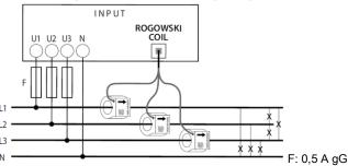
. Rogowski coil(s) cable length (see § Overall Dimensions) allow you to put Nemo SX Measure modules everywhere in the installation. This is not mandatory to have them near to the associated protection device of the measured line.
