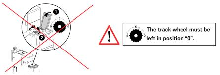
. It is not necessary to assign an address via rotary; **The track wheel must be left in default position "0**".
