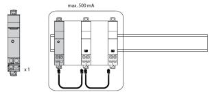
In this case is necessary to separate the two groups of devices with the decoupling white cable (delivered with the Nemo SX Power supply module)
