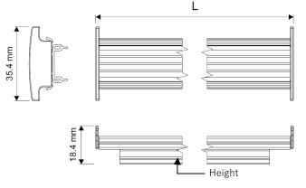
without the height spacer for mounting on DIN rails 7,5 mm depth
