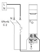
. Power supply protected by a Fuse holder:
