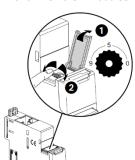
. Marked from 0 to 9 in order to locally define the Modbus address to Nemo SX modules In this system the Modbus address of a Nemo SX Nemo SX module device or group of modules (several functions) is obtained considering the address of the interface Modbus/Nemo SX Interface as tenth and the address of a device or group of function as unit (e.g. Interface address  $1 = 10 \rightarrow \text{address}$  of module  $n^{\circ}5 = \text{Modbus}$  address 15)
