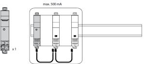
In this case is necessary to separate the two groups of devices with the decoupling white cable (delivered with the Nemo SX Power supply module)
