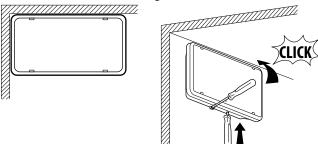
🗥 Can be unlocked using a screwdriver, minimum length 150 mm.
