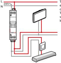
The branch can be joined in the electric cabinet, on the switch or in a junction box. The power supply to the units is subject to the same rule as the luminaires (normal wiring).
