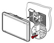
Positioning the 2 screws in the flush-mounting box.
