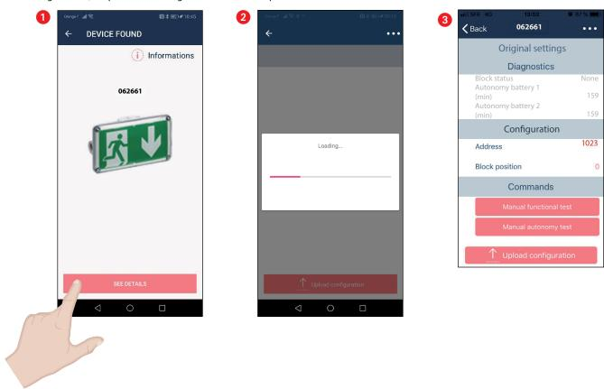
Step 4: In the "Diagnostics" part the user can see if the unit is faulty and the battery autonomy.
