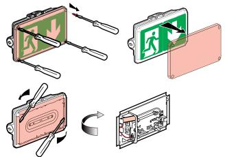
The batteries must be replaced when the self-contained unit can no longer provide its rated operating time.
