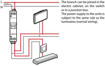
electric cabinet, on the switch or in a junction box. The power supply to the units is subject to the same rule as the luminaires (normal wiring).
