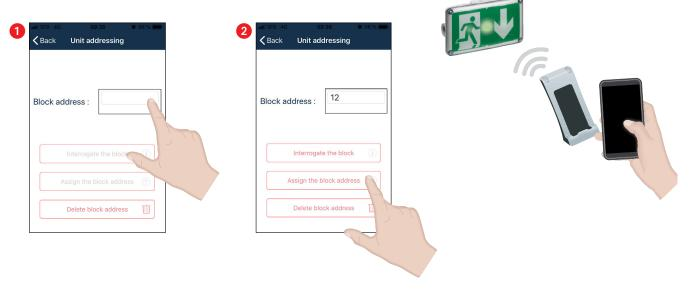
Assign an address number, then complete the action with **"Assign address to unit"**.
