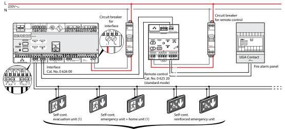
Max. length of a lighting unit line: 700 m. Above this length, place a repeater in series with the following lighting units
