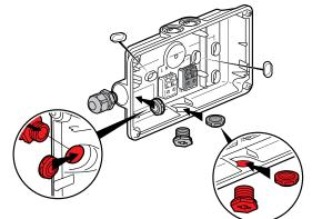
**Caution:** Ensure the nut is fitted the right way round, as shown above As soon as installation is complete, attach a maintenance label Cat. No. 0 609 00 and write the commissioning date on it (see 5.1) Attach the adhesive separable signalling label (supplied with the unit)
