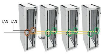
Deployment illustration with one daisy-chain on feed A and one daisy-chain on feed B
