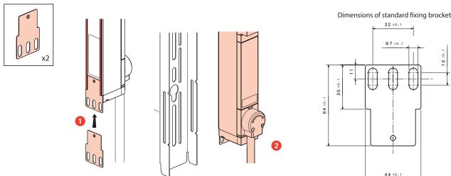
Fixing centres (min.-max.) with standard brackets : 1268mm -1288mm
