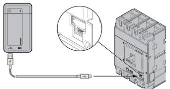
The cable to be used must be USB-Mini Type B with Megatiker switches or USB-Micro Type B with DMX3 MPX.10 switches.
