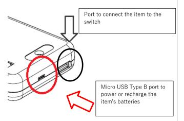
How to recharge the batteries or connect the dongle to an external power source
