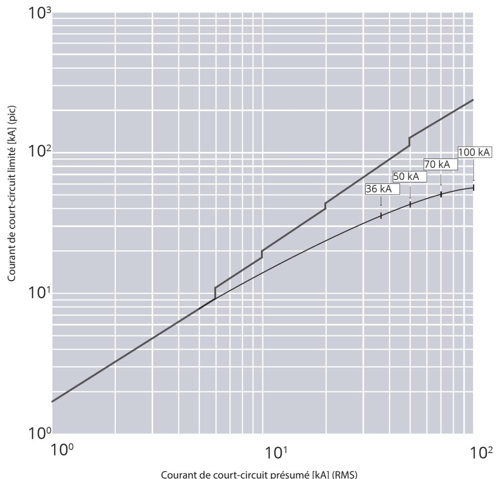
$I_{cu} = 36 - 50 - 70 - 100 \text{ kA}$     $I_{max} = 1600 \text{ A}$    3 - 4 P    $U_e = 415 \text{ V} \sim$  (IEC/EN 60947-2)
