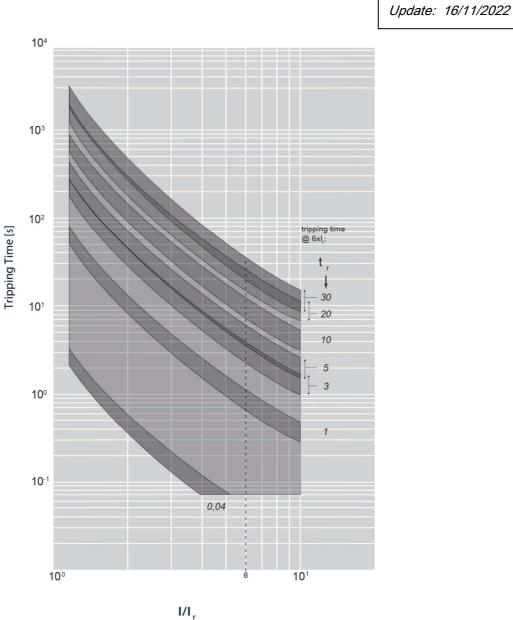
$I_{cu}$  = 36-50-70-100 kA  $I_{max}$  = 1600A 3-4 P  $U_{e}$  = 415Vac (IEC/EN 60947-2)
