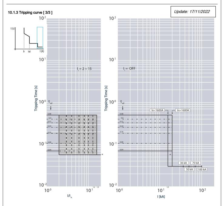
$I_{cu}$  = 36-50-70-100 kA  $I_{max}$  = 1600A 3-4 P  $U_{e}$  = 415Vac (/EC/EN 60947-2) Fixed Instantaneous override  $I_{sf}$  = 15kA (for  $I_{n}$  < 1600A) and  $I_{sf}$  = 20kA (for  $I_{n}$  =1600A)
