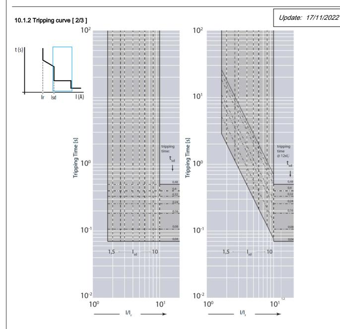
$I_{cu}$  = 36-50-70-100 kA  $I_{max}$  = 1600A 3-4 P  $U_{e}$  = 415Vac (IEC/EN 60947-2)
