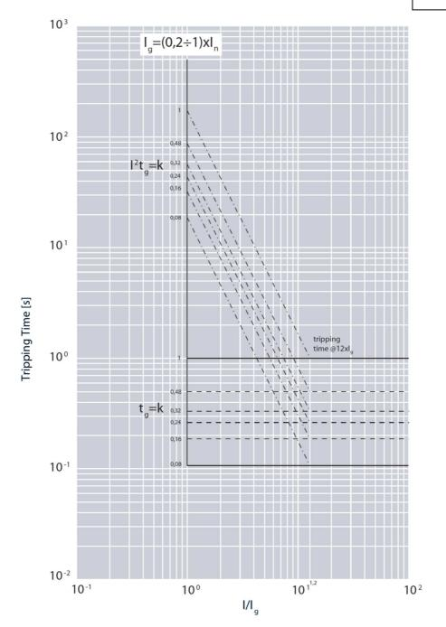
$I_{cu}$  = 36-50-70-100 kA  $I_{max}$  = 1600A 3-4 P  $U_{e}$  = 415Vac (IEC/EN 60947-2)
