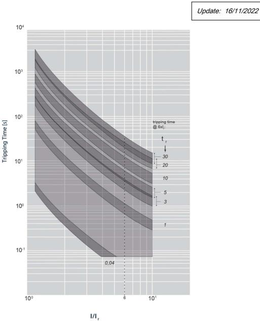
I<sub>cu</sub> = 36-50-70-100 kA I<sub>max</sub> = 1600A 3-4 P U<sub>e</sub> = 415Vac (IEC/EN 60947-2)
