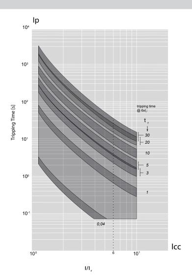
lcu = 36-50-70-100 kA lmax = 630 A 3-4 P  $Ue = 415 \text{V} \sim (IEC/EN 60947-2)$
