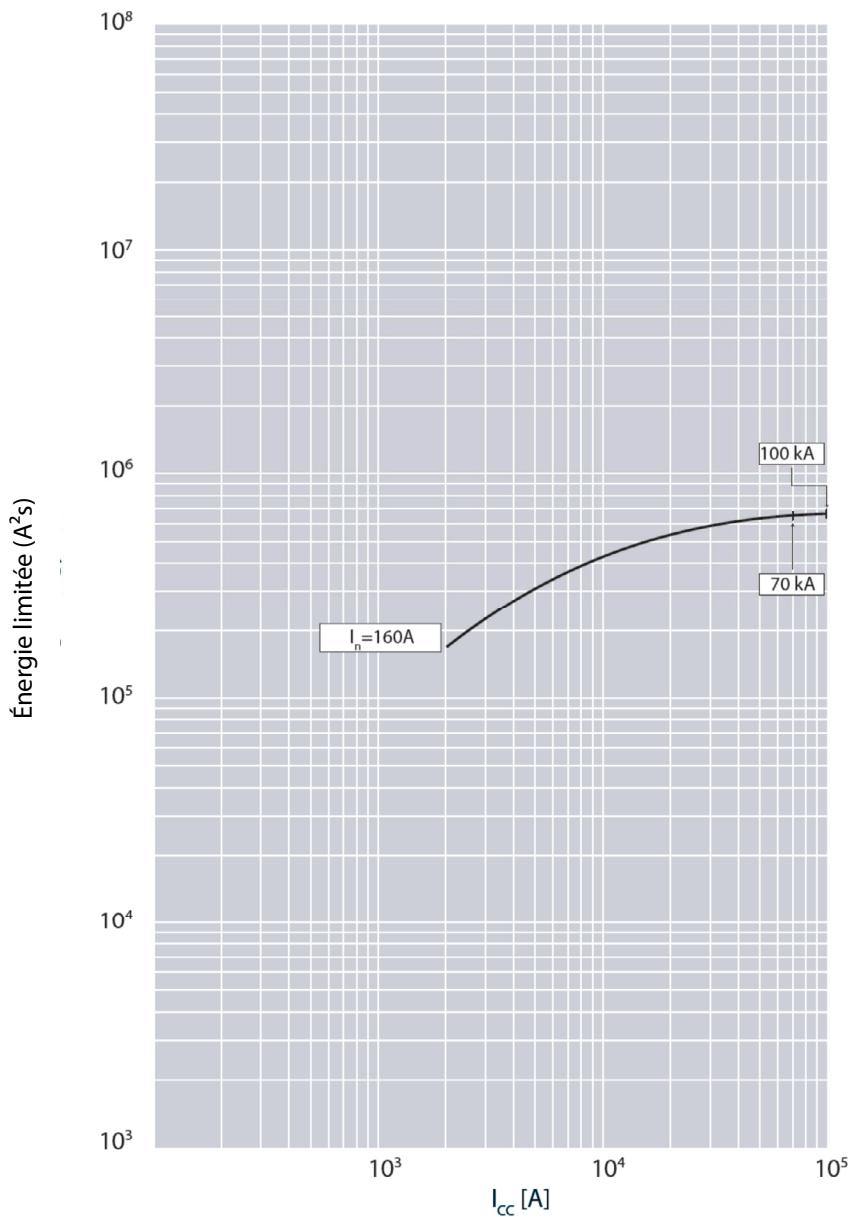
$I_{cu} = 36-50 \text{ kA}$     $I_{max} = 160 \text{ A}$    3-4 P    $U_e = 415 \text{ V}\sim$  (IEC/EN 60947-2)
