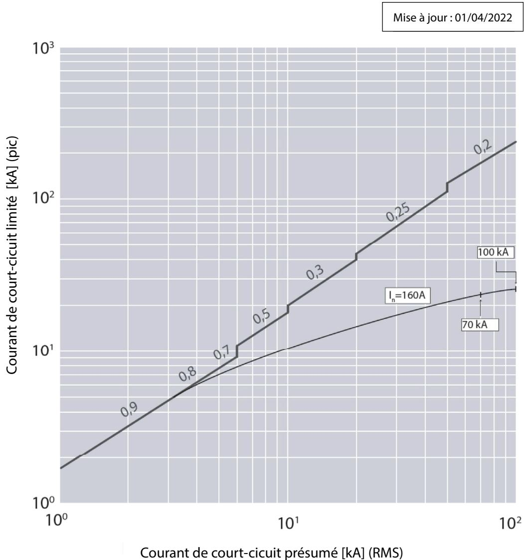
I<sub>cu</sub> = 70-100 kA      I<sub>max</sub> = 160 A      3-4 P      U<sub>e</sub> = 415 V~ (IEC/EN 60947-2)
