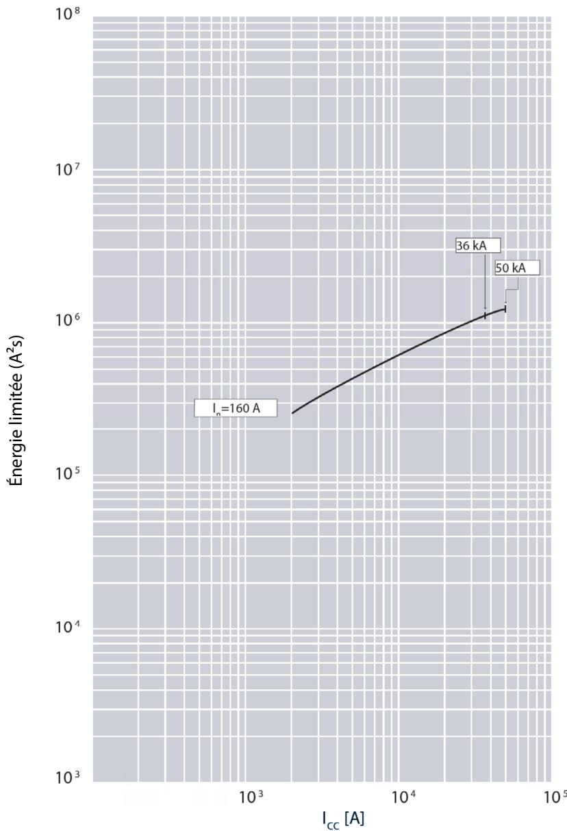
I<sub>cu</sub> = 36-50 kA      I<sub>max</sub> = 160 A      3-4 P      U<sub>e</sub> = 415 V~ (IEC/EN 60947-2)
