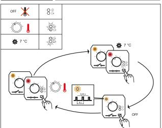
The external probe is used to limit the temperature in the floor.
