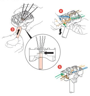
Spreading cables ensures that each pair is separated by the specified 13 mm.
