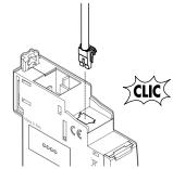
If necessary, use a small screwdriver on the clips to disconnect it.
