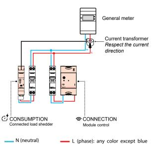
In a photovoltaic installation, the load shedding device cannot operate alone. It provides the total measurement (consumption part), while the photovoltaic measurement function (production part) is managed by a single-phase energy meter "with Netatmo" (refer to the technical documentation).
