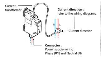
Wire the connected load shedder after a C2 to C16 protection circuit breaker according to the cable section used.
