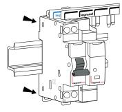
2. Pull the device forward to release it from the rail.
