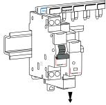
3. Pull the device downwards to fully disengage it from the comb teeth.
