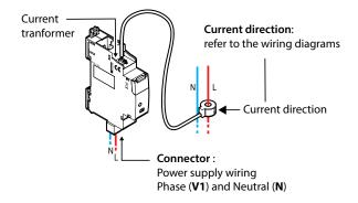
Wire the connected energy meter after a C2 to C16 protection circuit breaker according to the cable section used.
