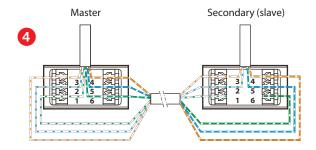
Spreading pairs at 90° to the cable ensures the best possible performance.
