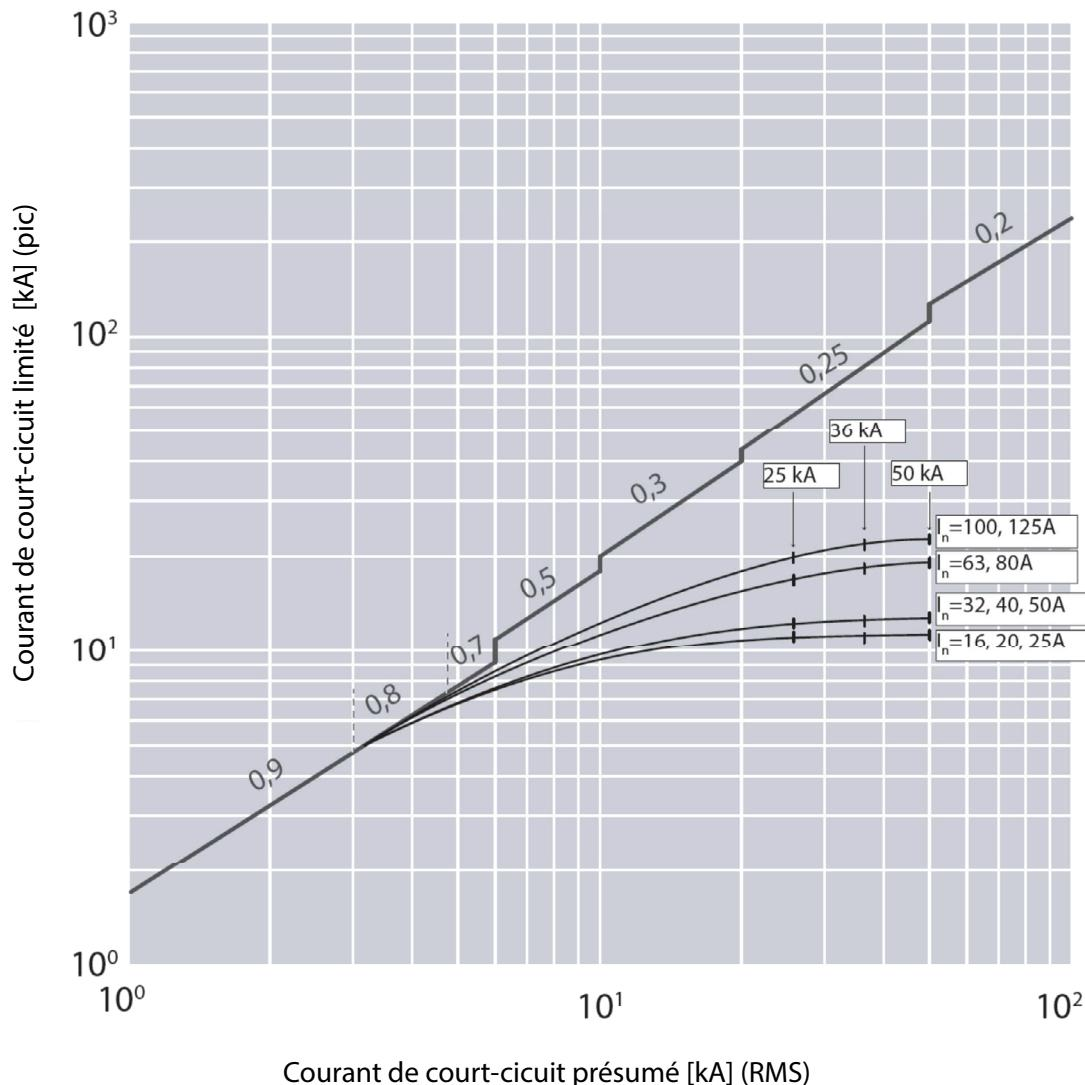
$I_{cu} = 36-50\text{ kA}$     $I_{max} = 125\text{ A}$    4P    $U_e = 415\text{ V}\sim$  (IEC/EN 60947-2)
