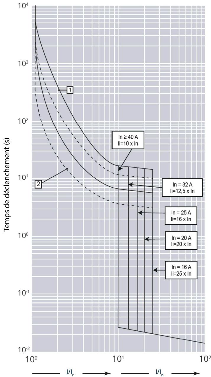
$I_{cu} = 36-50\text{ kA}$     $I_{max} = 125\text{ A}$    4P    $U_e = 415\text{ V}\sim$  (IEC/EN 60947-2)
