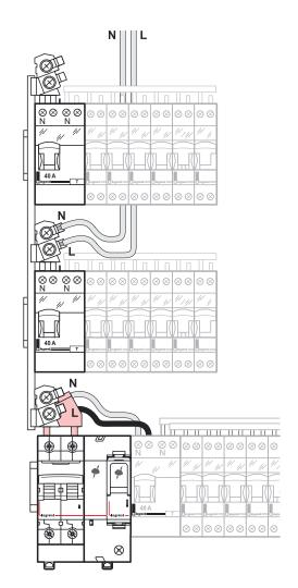
Mounting on lower rail with vertical supply busbars VX³ - 63A center distance 125 mm
