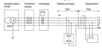
P1: main protective device of the installation If P1  $\leq$  C25 then choose a SPD without integrated lcc protection (4 122 24/25/26/27/44/45/46/47)
