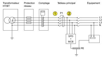
P1: main protective device of the installation If P1  $\leq$  C25 then choose a SPD without integrated lcc protection (4 122 24/25/26/27/44/45/46/47)
