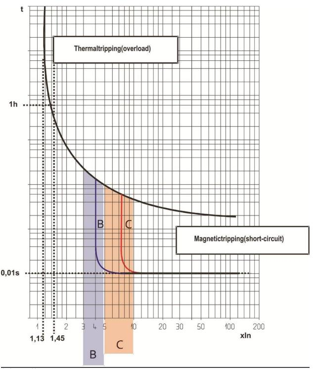
Thermal tripping at ambient temperature = 30°C In = DX³ STOP ARC rated current
