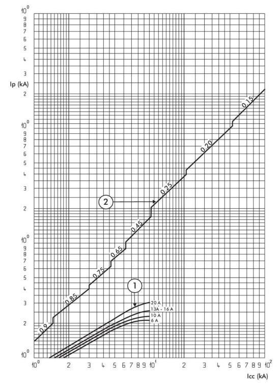
Icc = Prospective short-circuit symmetrical current (rms value in kA)
