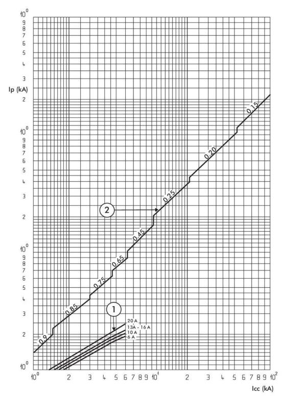
Icc = Prospective short-circuit symmetrical current (rms value in kA)
