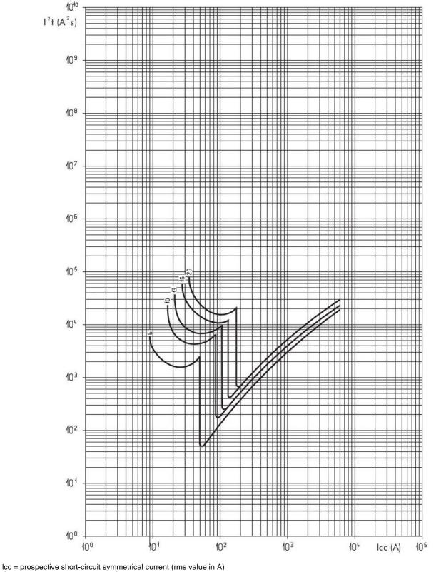
$I^{2}t$  = limited thermal stress (in A s)<sup>2</sup>
