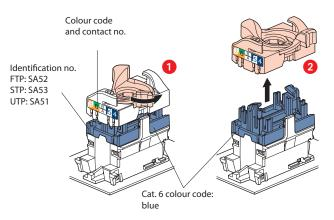
This system makes it easy to spread pairs before fitting them onto the connector
