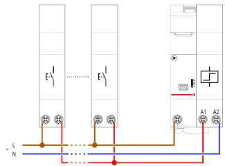
Control of a Contactor creating, with a Changeover switch - 2-way (e.g. cat. no 4 129 00), a local/remote command selector
