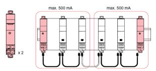
Note: in a system (beneath an EMS  $CX^3$ /Modbus interface) it is possible to use a maximum of 3 power supply modules = 3 groups of 500 mA.
