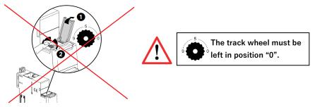
It is not necessary to assign an address via rotary, the track wheel must be left in default position "0".
