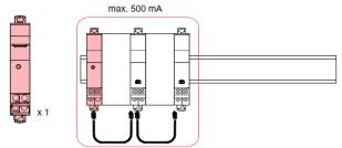
In this case is necessary to separate the two groups of devices with the decoupling white cable (delivered with the EMS  $CX^3$  Power supply module)
