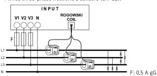
. Rogowski coil(s) cable length (see § Overall Dimensions) allow you to put EMS CX3 Measure modules everywhere in the installation. This is not mandatory to have them near to the associated protection device of the measured line.
