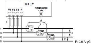
. Rogowski coil(s) cable length (see § Overall Dimensions) allow you to put EMS CX<sup>3</sup> Measure modules everywhere in the installation. This is not mandatory to have them near to the associated protection device of the measured line.
