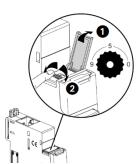
. Marked from 0 to 9 in order to locally define the Modbus address to EMS CX³ modules In this system the Modbus address of an EMS CX³ module device or group of modules (several functions) is obtained considering the address of the interface Modbus/EMS CX³ Interface as tenth and the address of a device or group of function as unit (e.g. Interface address  $1 = 10 \rightarrow$  address of module n° 5 = Modbus address 15)
