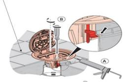
(6) Connect the mechanism with the cable. Don't forget the earth link.
