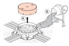
(2) Before installation of the back box, broke the protection cover (A) , and remove the last plastic parts (B)
