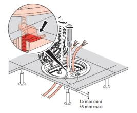
(4) Connect the mechanism with the cable. Don't forget the earth link
