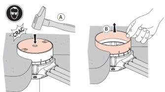
(3) Drill the back of the floor box at 20mm (A) and add the cable protection (B)
