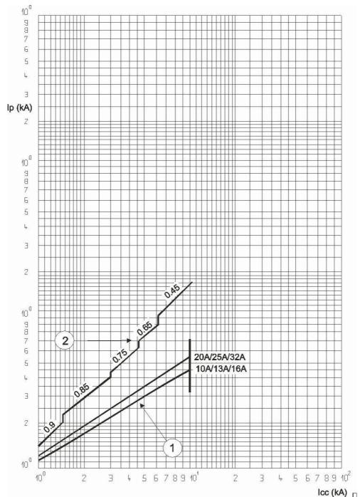
lcc = Prospective short-circuit symmetrical current (rms value in kA)
