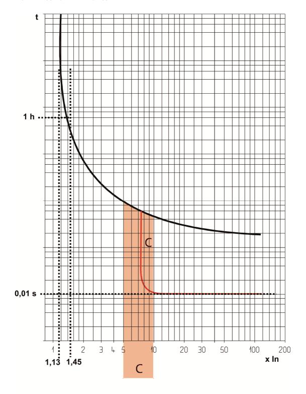
Thermal tripping at ambient temperature =  $30^{\circ}$ C In = RCBO rated current
