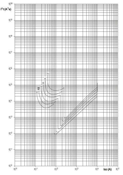
Icc = Prospective short-circuit symmetrical current (rms value in kA) I<sup>2</sup>t = Limited thermal stress (in A<sup>2</sup>s)
