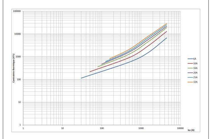
Icc = prospective short-circuit symmetrical current (rms value in A)
