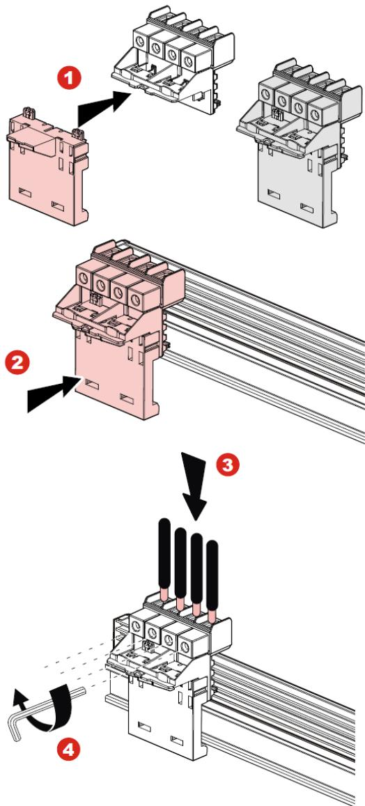
Supply module - Terminal capacity:
